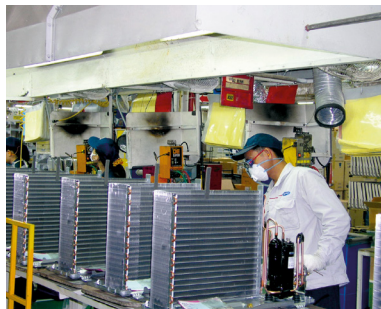
Outdoor units production
